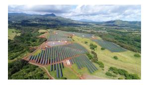
The AES facility in Lāwa'i features a 20 megawatt solar array with battery storage to facilitate a five-hour duration dispatch during evening peak *Photo credit: AES Distributed Energy*
