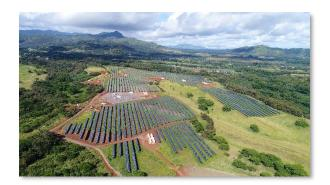
The AES Lāwa'i solar-plus-storage facility can provide up to 20 megawatts of direct-to-grid power during the day, along with five hours or 100 megawatt hours of electricity for use after sunset. *Photo credit: AES*
